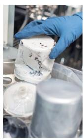
stage cleaning process with automated pre- and post-cleaning. Just 5 litres of KANCLEAN cleaning fluid are needed for about 100 cups and lids. This water based paint cleaner, specially developed for this application, convinces with its residue-free washing results, even with dried water based paints. Additionally, KANDO offers an amazing cost-saving potential combined with convincing cleaning results.
